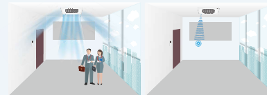
The indoor unit automatically runs when detecting human body. The indoor unit automatically stops when detecting absence.
