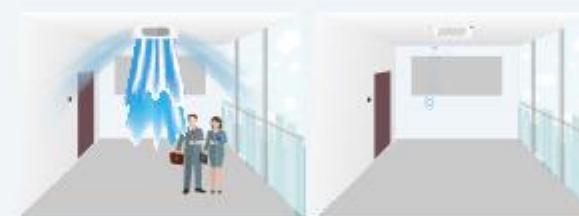
The indoor unit automatically runs when detecting human body The indoor unit automatically stops when detecting absence
